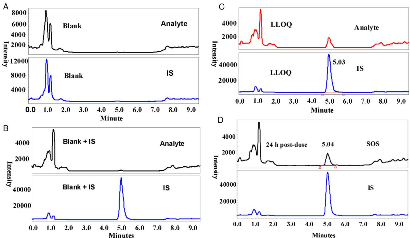
Fig. 2. LC–MS/MS chromatograms of (a) blank dog plasma (b) blank dog plasma with internal standard  $^{13}\text{C}_{12}$ -sucrose octasulfate (c) spiked LLOQ of sucrose octasulfate in dog  $\text{K}_2\text{EDTA}$  plasma and (d) a  $\text{K}_2\text{EDTA}$  dog plasma sample of post-dose after 24 h.
